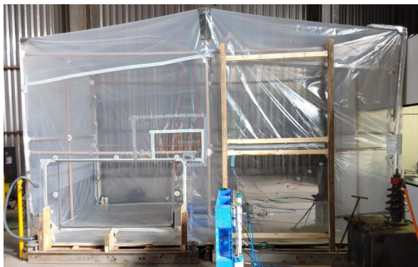
Figure 3: External view of the salt-fog chamber.
