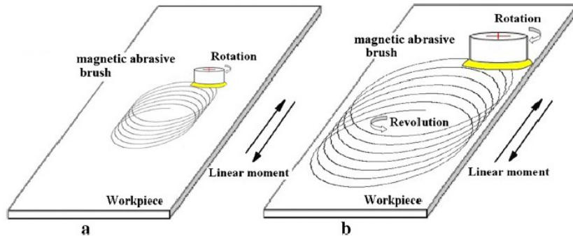
**Figure 3:** a – Conventional trajectory of magnetic finishing; b – Enhanced trajectory.
