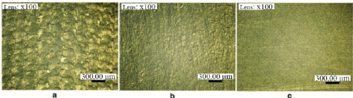
**Figure 2:** a – Surface of a titanium workpiece after milling. b – Surface of a titanium workpiece after magnetic abrasive finishing. c – Surface of a titanium workpiece after ultrasonic vibration assisted magnetic abrasive finishing.
