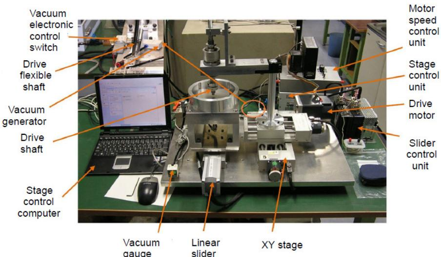
**Figure 4:** Prototype developed to carry out the enhancement tests of trajectory in magnetic abrasive polishing.
