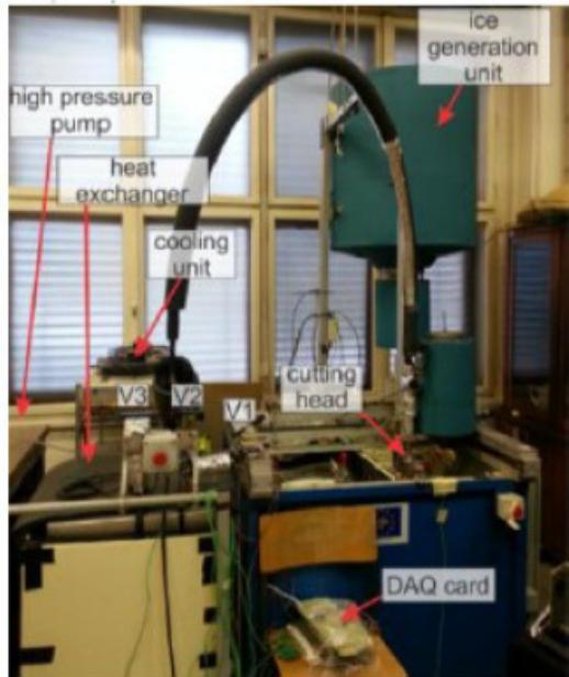
**Figure 5:** Water jet machine adapted to tests of IAWJ.
