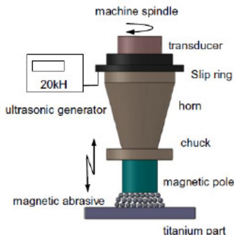
**Figure 1:** Schematization of the tool used in ultrasonic assisted magnetic abrasive finishing process.
